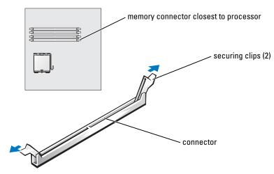
4 Align the notch on the bottom of the module with the crossbar in the connector.
