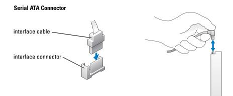
Most interface connectors are keyed for correct insertion; that is, a notch or a missing pin on one connector matches a tab or a filled-in hole on the other connector.
