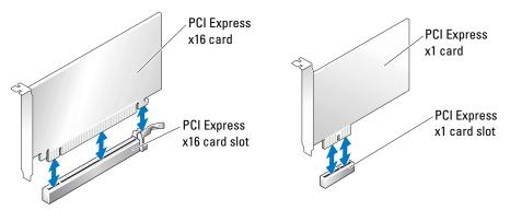
If you are installing or replacing a PCI Express card, follow the procedures in the next section. If you are removing but not replacing a card, see "Removing a PCI Express Card" on page 85. If you are replacing a card, remove the current driver for the card from the operating system. If you are installing or replacing a PCI card, see "Installing a PCI Card" on page 76.
