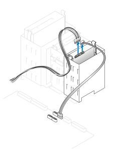
2 Press in on the tabs on each side of the drive and slide the drive up and out.
