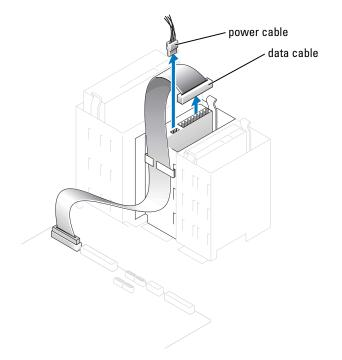
**3** Press inward on the two tabs on the sides of the drive, slide the drive upward, and then remove it from the floppy-drive bay.
