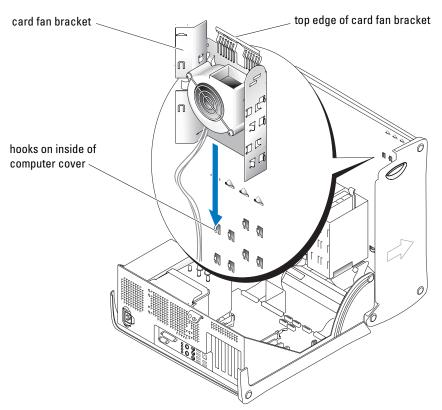
**3** Slide the card fan bracket onto the hooks on the inside of the computer cover.
